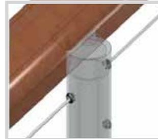
PICTURE: GROM-B37 grommets installed on a 37° stair angle post.
